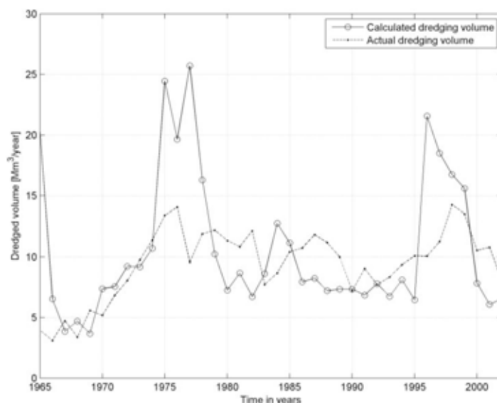
Figure 6. Calculated and actual total dredging amount per year for the entire Western Scheldt for 1965-2002
